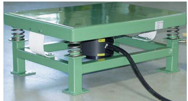
Compaction of powder in sacks
